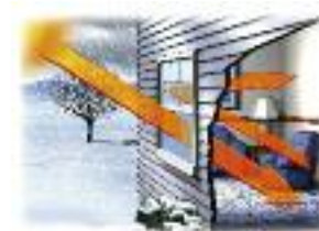
In winter months, Low-E glass lets warm solar rays into your home, while preventing indoor heat from escaping.
